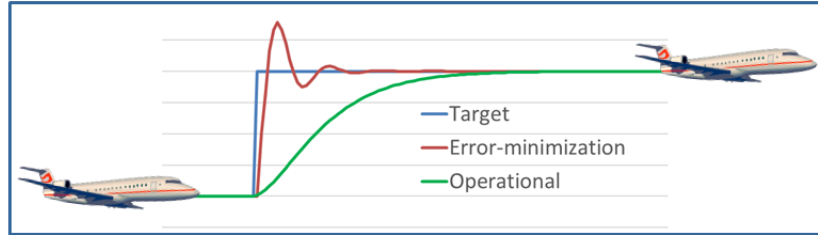
Figure 3: The analogy of a passenger plane changing altitude illustrates why 'operational performance' criteria are more appropriate for industrial process operation than traditional model-based error-minimization.
